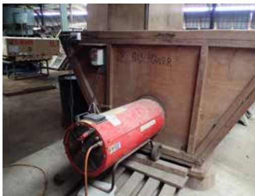
Jet blast air dryer for effective sea cucumbers drying.
